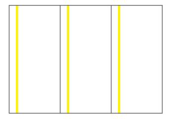
Product edges are precisely cut in order to use butt joint (edge to edge). Overlap is not recommended for woven styles, but can be used for nonwoven products (veils). When matching adjacent panels together, respect the pattern weaving in order to make joint "invisible".
